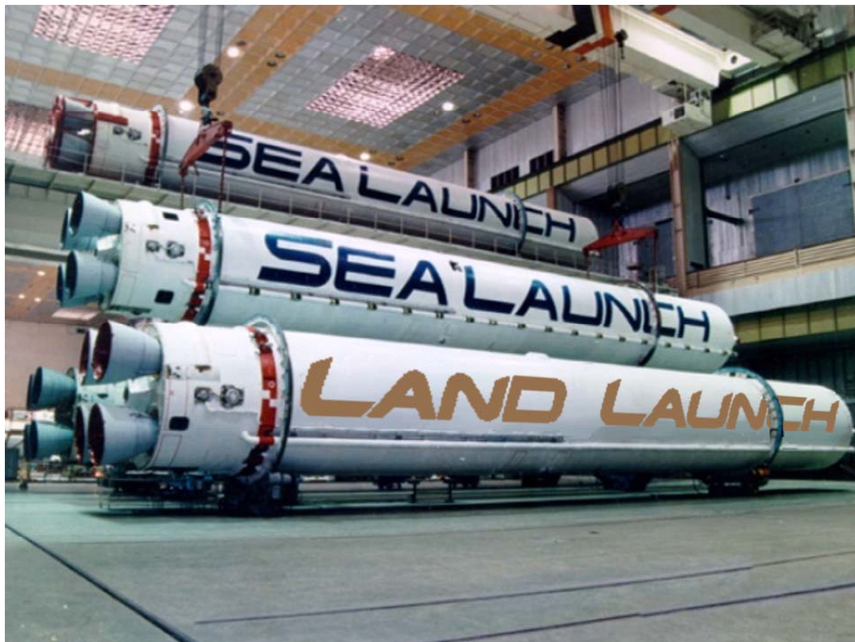
Figure 2-5. PO Yuzhmash Achieves Significant Economies of Scale by Manufacturing Both Land Launch and Sea Launch Zenit Stages on the Same Production Line
